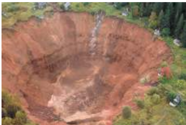
Fig. 3.2.16. Technogenic karst failure in the territory of suburban areas, Solikamsk, Russia: a – 2014; b – 2016; c – 2018
