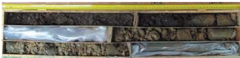
Fig. 5.4.7. Drilled coring in volcanic weathered basalt
