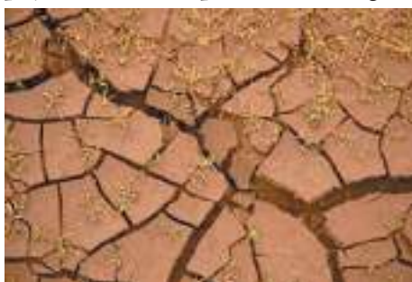
Fig. 4.6.6. Shrinkage of swelling soils during drying
