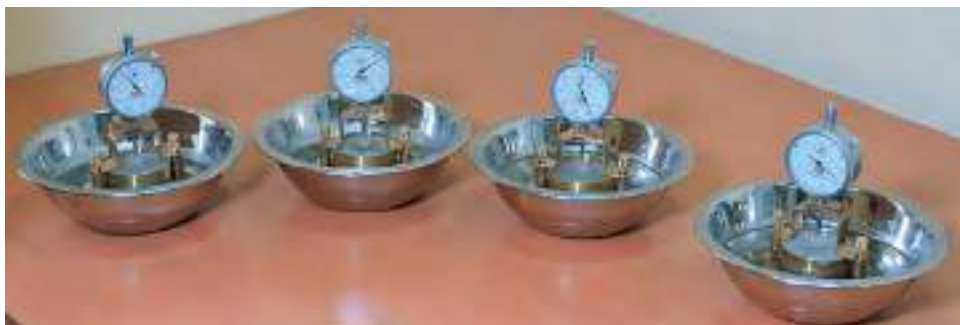
Fig. 4.6.8. Testing swellable soils
