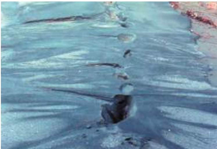
Fig. 3.10.17. Sand Boils, Loma Prieta, SF, USA 1989 http://www.maipark.com/assets/uploads/Erly.pd
